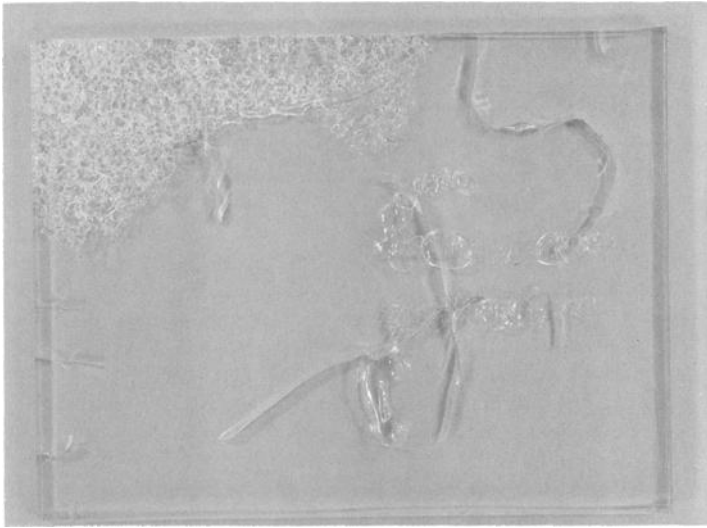
FIG. 4—9.27 mm plate glass heated to 450°C for 30 min prior to removal from the furnace. Crazed area was sprayed with water.
